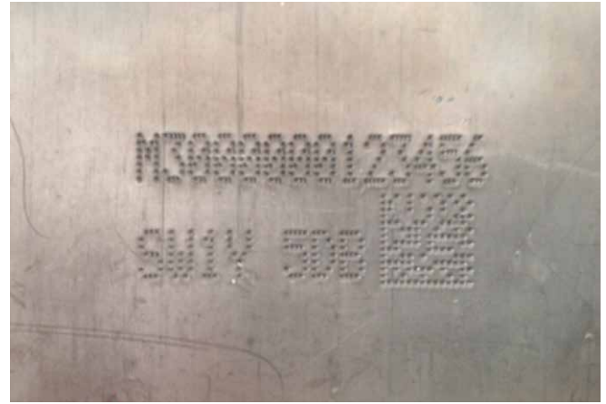
Figure 23 Example of identifying markings which can be made on metal.
